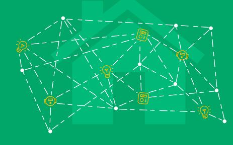
Similarly, Zigbee devices can be easily commissioned to communicate with each other using a mesh network to share information.
