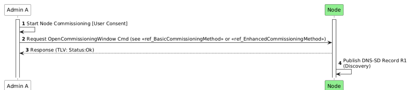
Figure 41. Open Commissioning Window (Administrator A)
